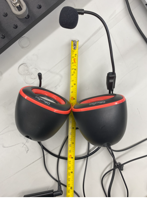
Fig. 1: Picture of the experimental setup to measure latency, impulse response, and frequency response of the speaker and microphone combination
